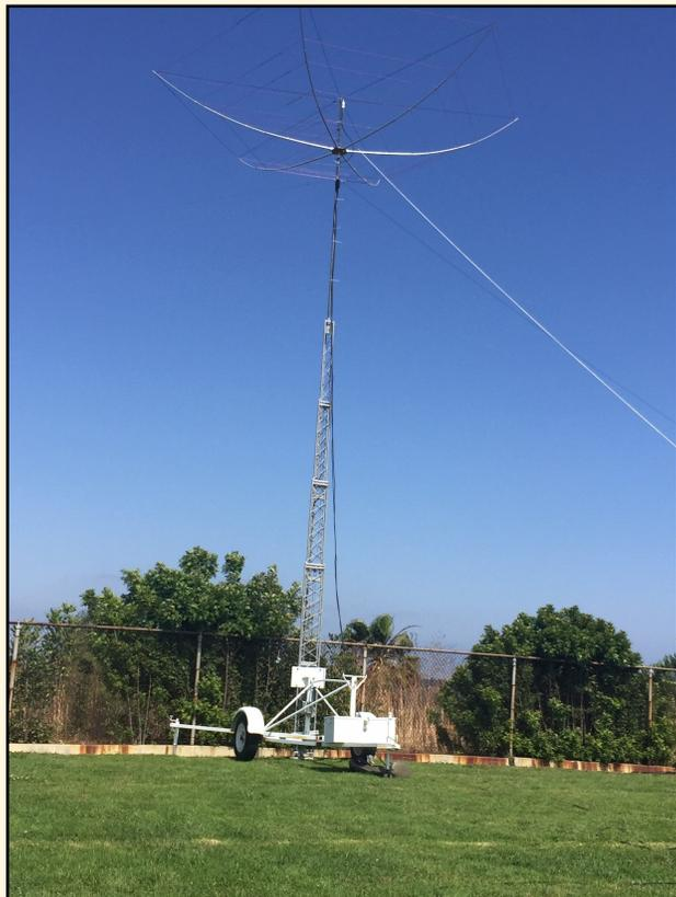
**K6PV Tower Trailer:** This year our CW, SSB, and FT8 stations operated from a common hexbeam and 80/40 wire dipoles with bandpass filters. This accelerated our setup on Saturday, with only three hours between initial site access and the 11 am start of contacts. PHOTO: MALIN DOLLINGER, KO6MD
