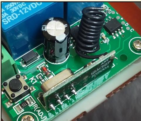
**Figure 2.** The tiny (1" x 2") UHF receiver circuit picks up signals from the key fob and activates the appropriate relay circuit.
