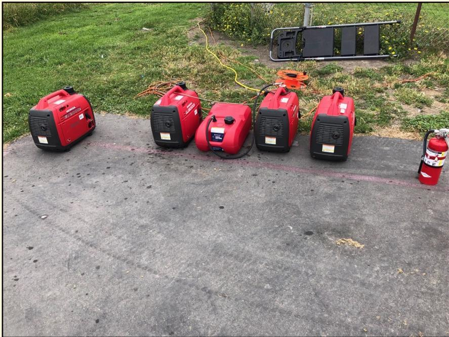
**Generator Alley:** Four compact Honda generators powered K6PV at Field Day, including the external fuel tank (center) of Jerry, NG6R, which allows continuous operation of up to 72 hours. PHOTO: GARY LOPES, WA6MEM
