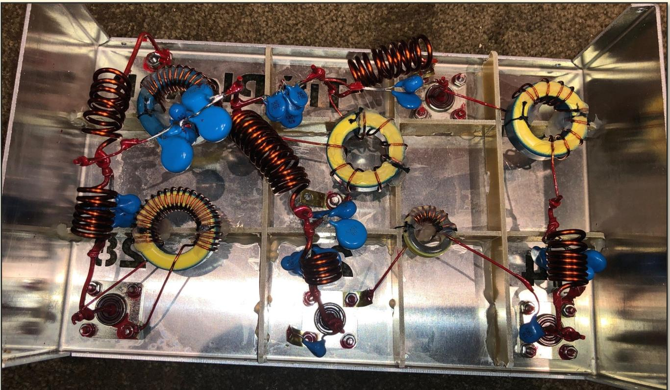
**Figure 5.** Top view of new 10m/15m/20m high power HF Triplexer. Note the point-to-point wiring on an elevated insulating grid support structure, as compared with the PCB approach of VA6AM's layout shown in Figures 1 and 2.
