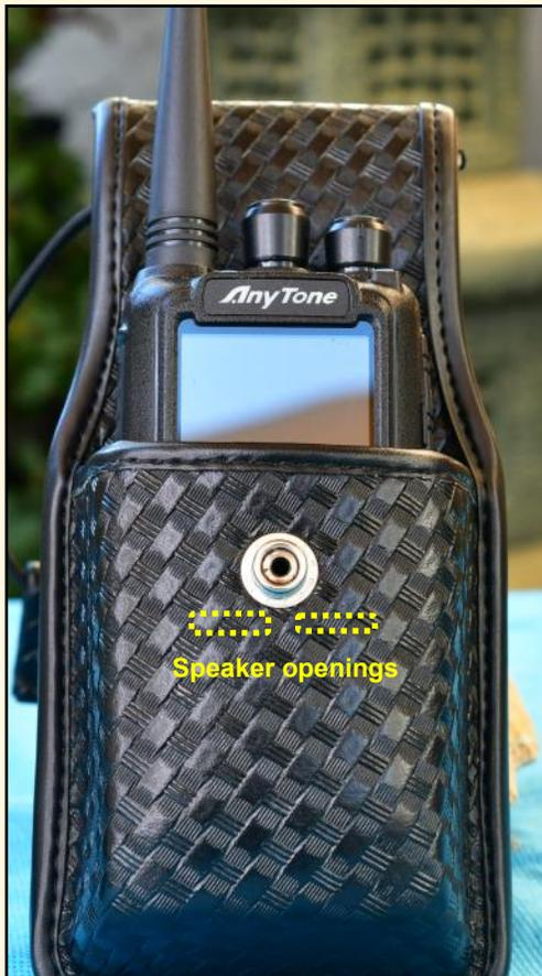
**Poor:** Display fully exposed to possible damage and speaker in center of radio is totally covered by holster...speaker mic needed with a holster.
