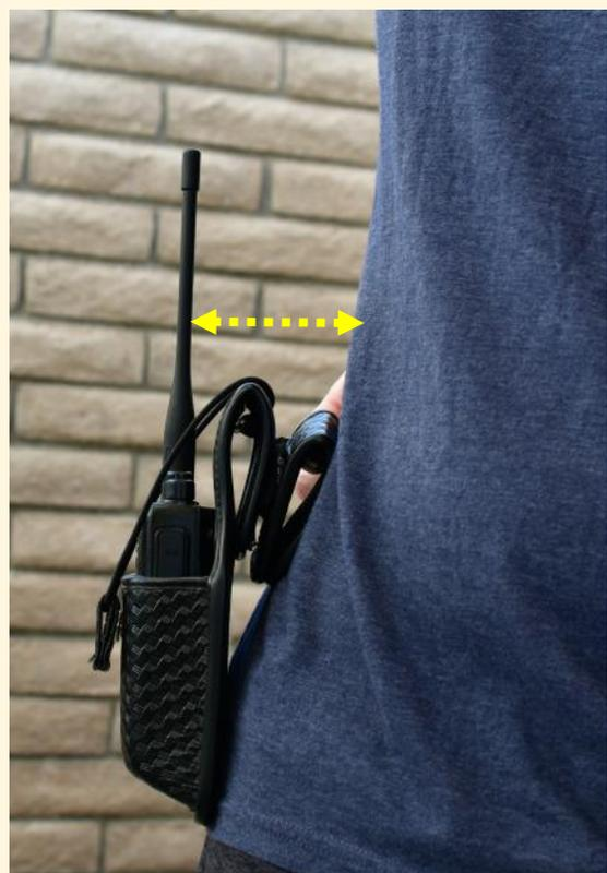
Radio holsters for public safety professionals do two things: they angle the antenna away from your body and the holster swivels when you sit down. The typical radio belt clip puts the antenna right next to your body and doesn't swivel.
