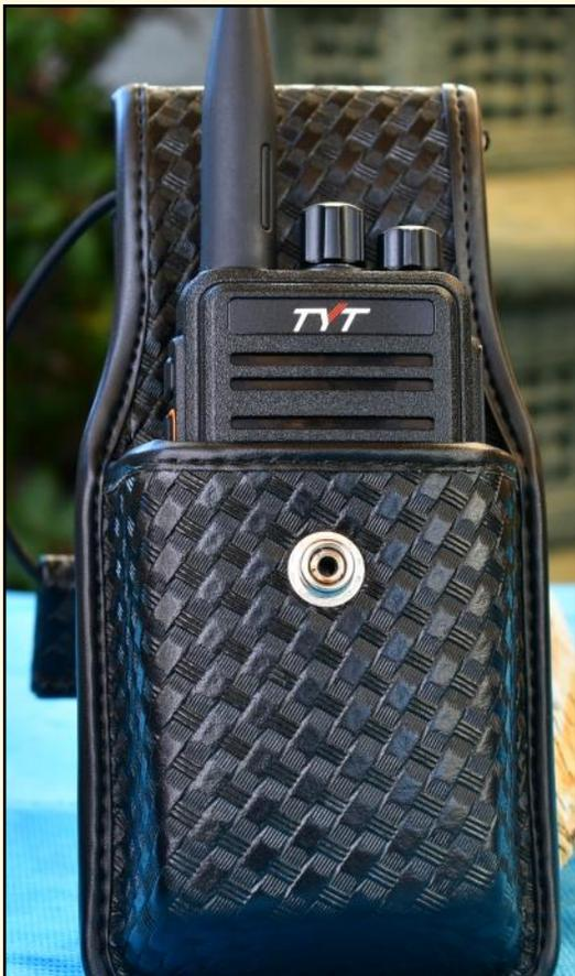
**Good:** Display is protected, speaker mostly open...but narrow spacing between top knobs makes for awkward finger access.
