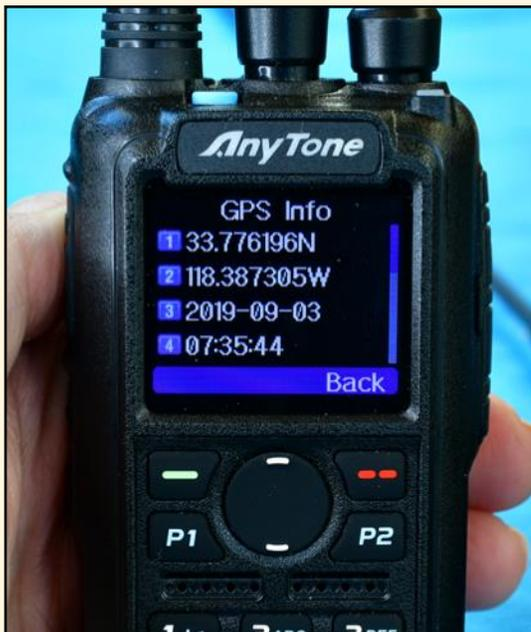
**Nice feature #1 on AnyTone 878UV:** Built-in GPS system works great but it's buried in the Menu options. Be advised: GPS screen only stays on for 10 seconds before reverting to home screen...if you haven't copied the coordinates by then you need to start all over through the Menus to reach the GPS.
