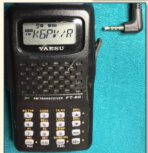
**Above:** It happens...Yaesu FT60 four-conductor combined plug for earpiece and PTT mic doesn’t have a secured seat in its jack—when it comes partially out (top) the PTT is closed, radio goes into transmit.
