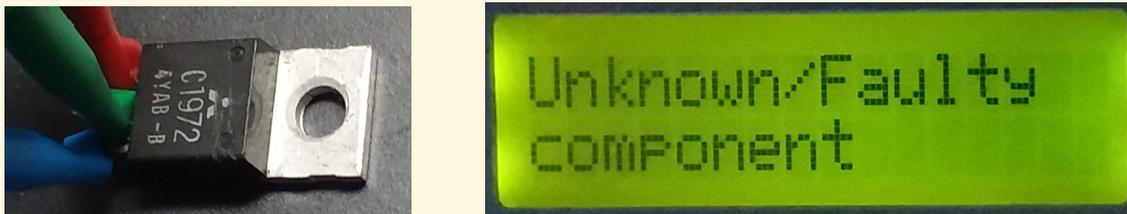
**Figure 4.** This Mitsubishi power transistor is known to have failed and was replaced. The failure mode was such that no additional information about the specific failure details can be discerned by the DCA55 tester. PHOTOS: JERRY KENDRICK, NG6R
