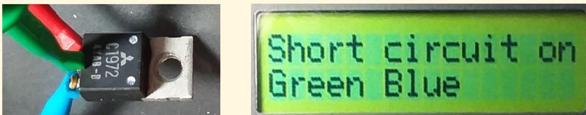
**Figure 5.** This second Mitsubishi power transistor, which failed and was replaced at the same time as example #3 above, indicates that a short exists between the collector (green) and emitter (blue). PHOTOS: JERRY KENDRICK, NG6R
