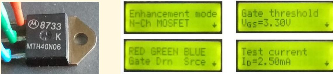
**Figure 3.** The Motorola MTH40N06 component was properly characterized as an enhancement mode N-channel MOSFET and its gate, drain and source terminals were correctly identified. Its gate threshold voltage value of 3.3V at a drain current of 2.5mA is in the range of acceptable voltage values (2.0V – 4.5V) shown in Reference [2]. PHOTOS: JERRY KENDRICK, NG6R
