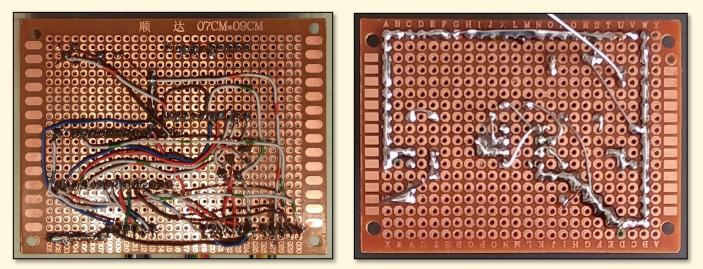
Figure 6. Rear interconnections of the Nano/DDS board (left) and the linear RF amplifier board (right). A continuous wire-embedded perimeter solder bridge is a convenient ground on the amplifier board.
