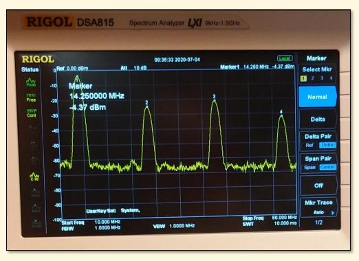
**Figure 7.** (Upper) A frequency of 14.25 MHz was selected with the front panel rotary encoder knob.
