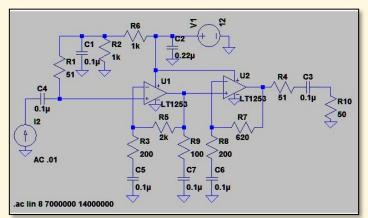
Prior to the decision to make, rather than buy, this amplifier, the schematic in Reference [11] was simulated using LTSpice. The SPICE simulation tool is very familiar and has been used for previous PVARC projects [12]. The simulation diagram is shown in Figure 3.
