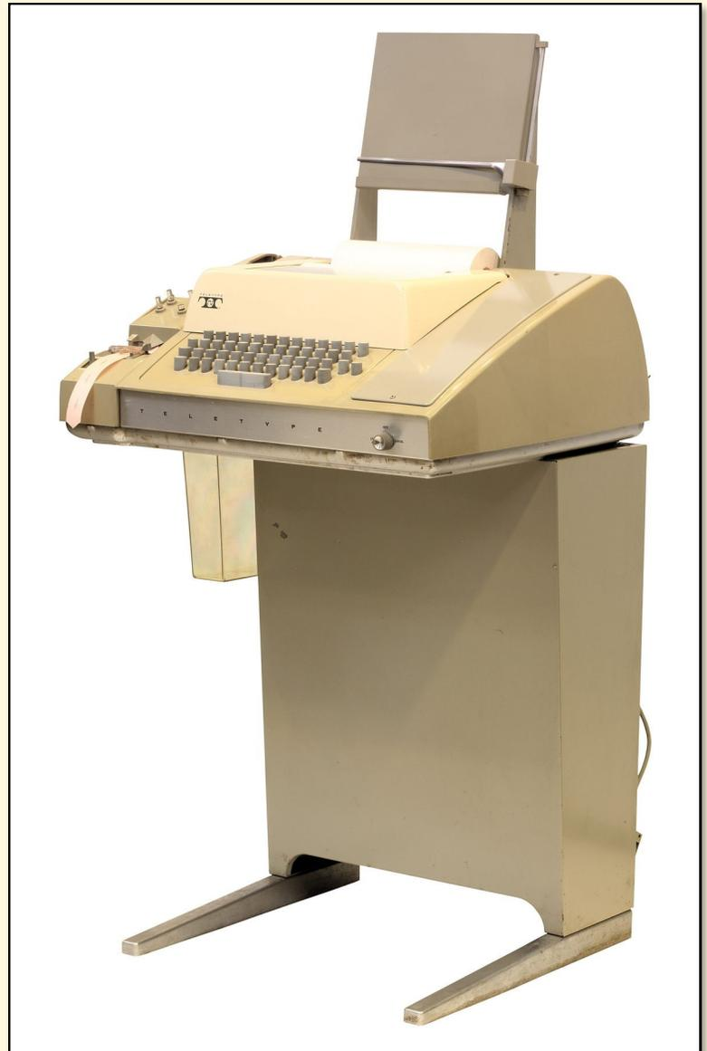
**Above:** ASR-33 Teletype on display at the Musée Bolo, EPFL, Lausanne, France. Some ham stations still use these 1970's machines with punched paper tapes for RTTY although most hams have migrated to RTTY software using computer soundcards.
