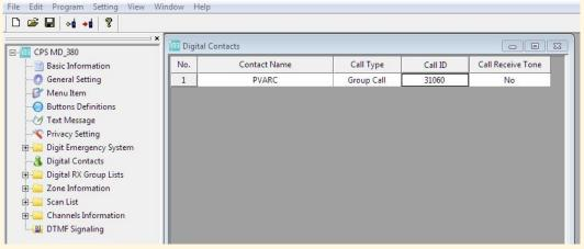
**Figure 4.** This is the single-entry "list" of contacts I've set up. There's just one for now and it's PVARC with its own TG designator: 31060.
