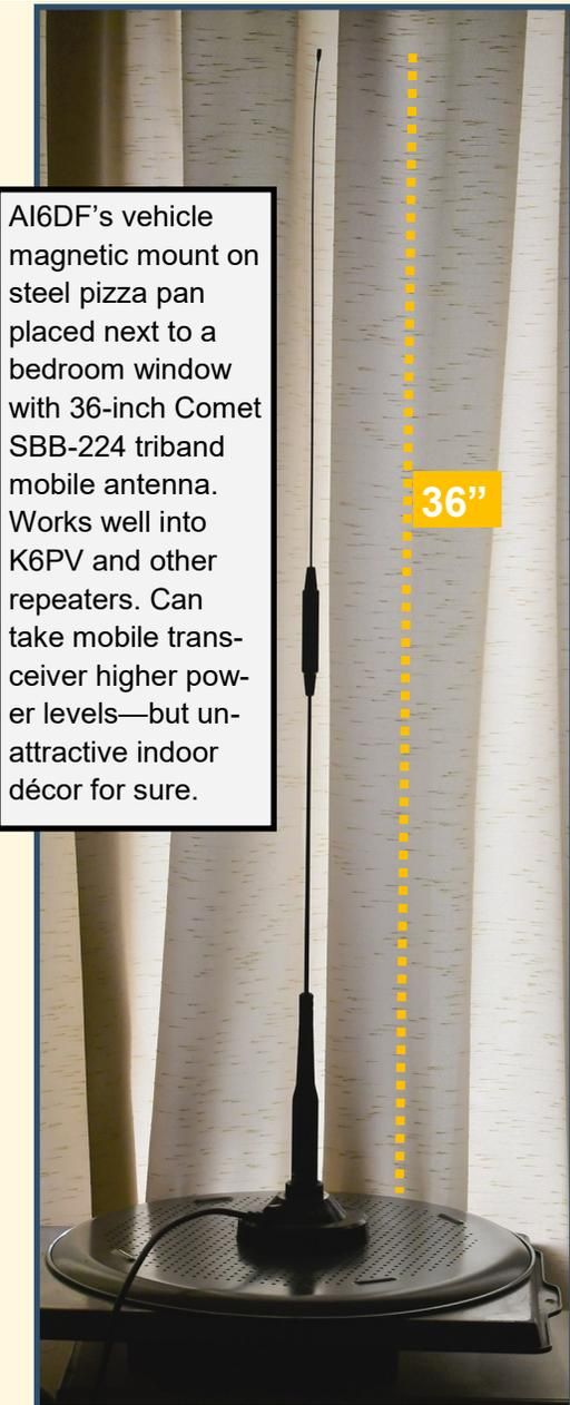
AI6DF's vehicle magnetic mount on steel pizza pan placed next to a bedroom window with 36-inch Comet SBB-224 triband mobile antenna. Works well into K6PV and other repeaters. Can take mobile transceiver higher power levels—but unattractive indoor décor for sure.
