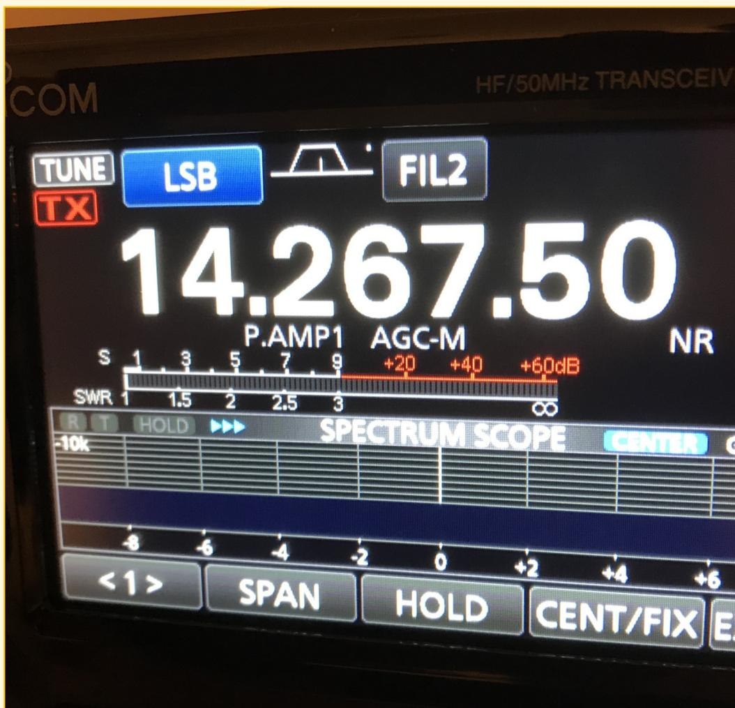
**Above:** Oops...LSB is the wrong convention for this frequency—on ham bands above 9 MHz and on 60-meters all single-sideband operation should be on upper sideband. Modern transceivers like this Icom IC-7300 enable selecting either LSB or USB on any SSB frequency...but it’s up to the operator to ensure using the proper convention. PHOTO: DIANA FEINBERG, AI6DF
