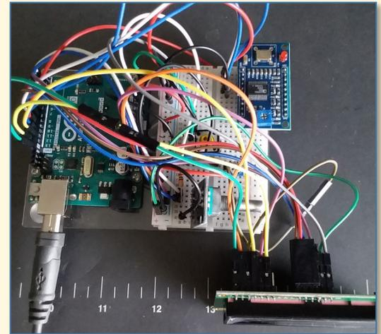
**Figure 2.** Author’s breadboard of four of the six components of the DDS VFO (less the homemade buffer amplifier and regulated voltage boards). An Arduino UNO was used in lieu of the smaller Nano, but it has similar pinouts. The USB cable in the lower left not only provides power for all active components via the Arduino 5V bus, but also provides the means for uploading the software program or “sketch” into the Arduino microcontroller.
