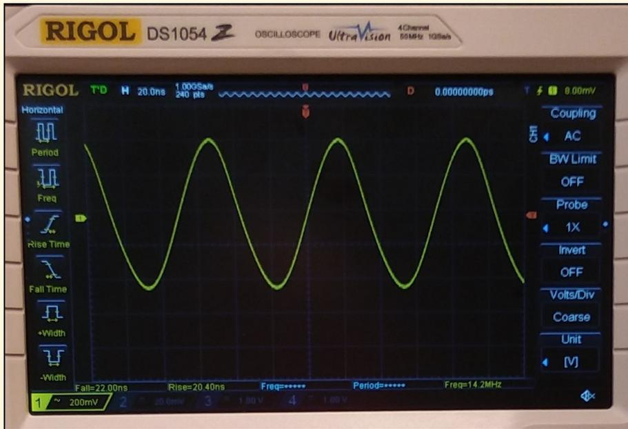
**Figure 7.** (Upper) A frequency of 14.25 MHz was selected with the front panel rotary encoder knob.
