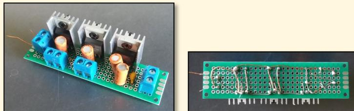
**Figure 5.** (Left) Schematic of the three-stage voltage regulator board; (Middle) overhead view of its realization in hardware; and (Right) rear of board showing thru-hole component interconnects. Heat sinks were added to eliminate some of the heat created in each of the regulator ICs.
