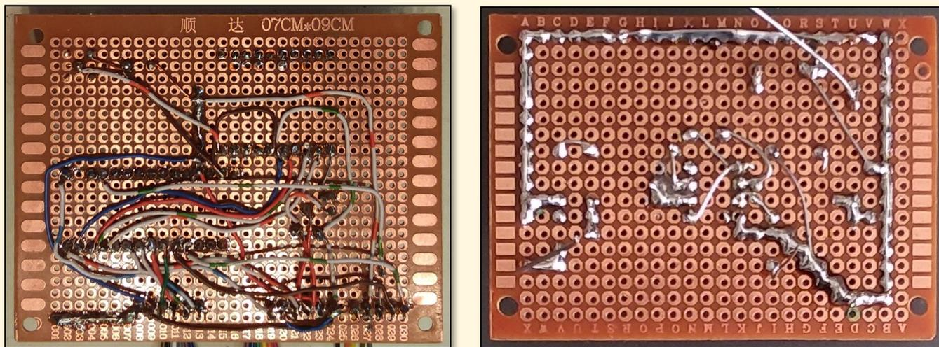
**Figure 6.** Rear interconnections of the Nano/DDS board (left) and the linear RF amplifier board (right). A continuous wire-embedded perimeter solder bridge is a convenient ground on the amplifier board.
