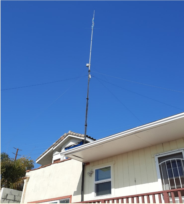
Cushcraft R4 vertical for 10/12/15/20m (40m inverted V dipole barely visible)
