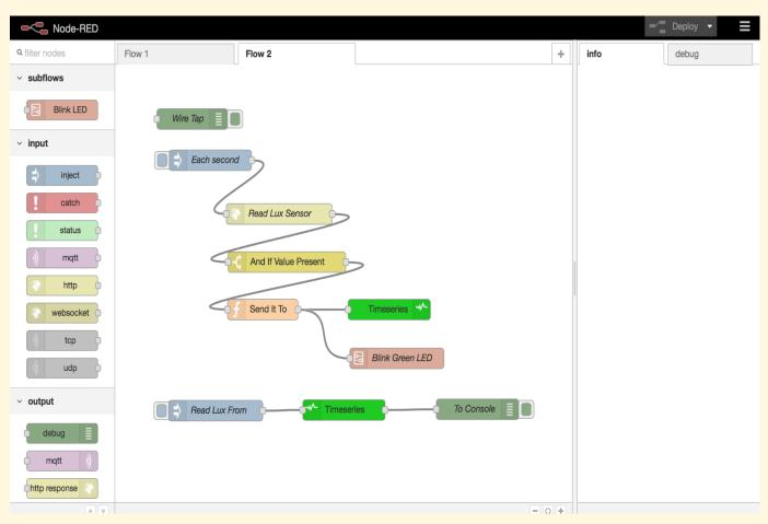
The Node-Red flow for controlling the K6PV repeater is more complex than the flow noted above but was developed using the same standard Node-Red modules to control the opening and closure of three relays. These relays individually switch the selected I/O pin to low (ground) or high (open) to complete the requested command.
