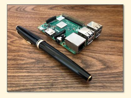
**Left:** Enabling remotely controlling the K6PV repeater mode (into Analog Only, DMR Only, or Mixed Mode) is the Raspberry Pi 3 Model B+, shown alongside a Mont Blanc pen to illustrate comparative size.
