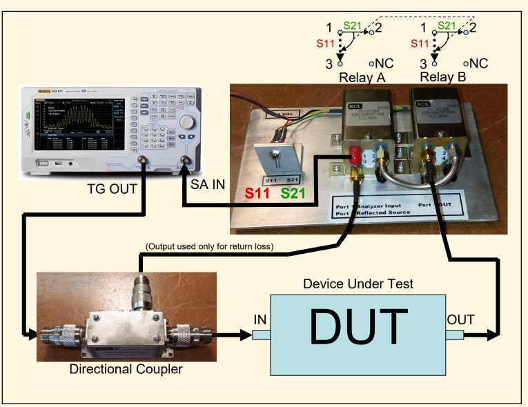
**Figure 3.** Schematic diagram of RF relay network. Configuration showing WA6MEM's automated RF relay switching platform, along with directional coupler and tracking-generator-equipped spectrum analyzer, to subject a device under test (DUT) to a measurement of both insertion loss and reflected loss with the simple throw of a switch. That switch can be seen on the switching platform, labeled S11 S21.
