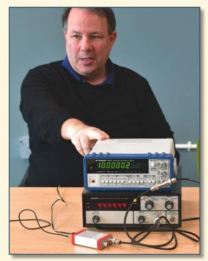
Above: Brian, K6BRN, discusses his BK and Heathkit temperature-compensated frequency counters. Below: AC6RM's palm-sized Soviet CW key. Bottom left: Ray, N6HE, made low-cost adapter for DB-15 connector to also handle HF radio accessory functions. Bottom right: Carlos, WD6Y, enhanced his Arduino electronic clock with GPS and weather functions. PHOTOS: DIANA FEINBERG, AI6DF
