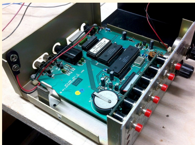
Figure 3. (Left) MFJ-492 with cover removed. Integrated circuit (IC) dominance on the horizontal PCB is obvious. Note the red button switches are on a separate vertically oriented PCB. All the external interface components are attached directly to the horizontal PCB (rear: RCA connectors for TX keying; ¼” stereo jack for CW paddle; 12V-15V DC power jack; and front: on/off power switch; speed and volume control variable resistors) (Right) The original embossed front panel with the 4x5 programming matrix was removed and discarded. The bulk of the original green PCB has been cut away and discarded to make room for the Arduino UNO that is secured to the bottom of the aluminum enclosure. Two small PCBs have also been added—one near the rear that contains an LM386 audio amplifier IC circuit; and one on the left side that houses five resistor/capacitor pairs acting as a low-pass filter to convert an output square wave tone signal (from the Arduino) to a near sine wave for improved tonal quality; and also contains a 4N33 optocoupler chip to key a transmitter (via the RCA jack at the rear) and yet isolate the Arduino from the external transmitter keying circuit.
