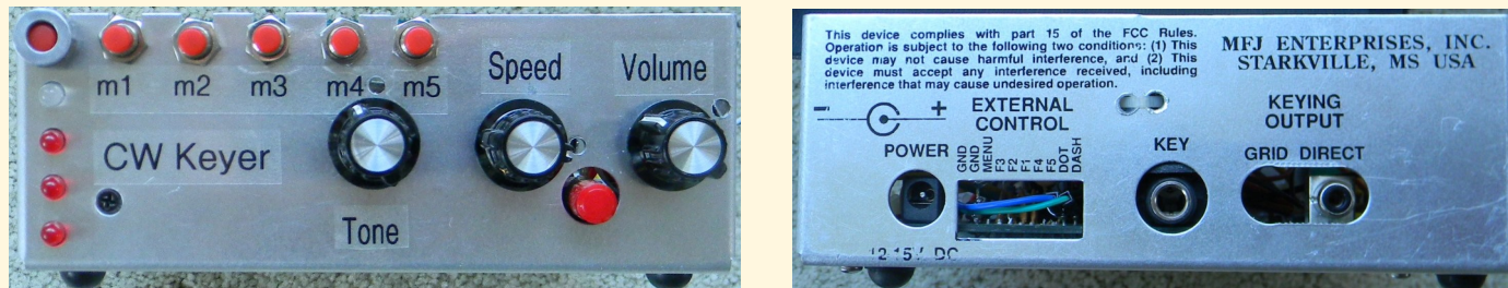
Figure 4. (Left) Front-panel view of repurposed CW Keyer. The top left red button switch is used to initiate programming of the five code sequence memories (m1 thru m5). Once programmed, a single push of a memory button will transmit the respective code sequence. (Right) Rear view of keyer showing intact connectors: 12V-15V DC power input, paddle key and direct TX keying output. Paddle dot/dash polarity can be reversed by simply interchanging the blue and green connector wires without having to remove the unit cover.
