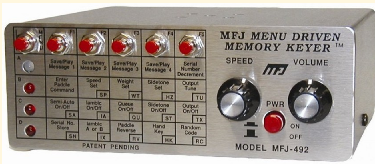
Figure 1. Front view of MFJ-492 menu driven memory CW keyer. It is controlled via a menu of options shown on the front panel by successively selecting a row with the top-left MENU button (confirmed by lighting a row LED) and then selecting a column with buttons F1 thru F5. There are rotatable controls for code speed and audio volume, as well as on/off power button, also accessible on the front panel.
