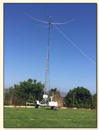
K6PV Tower Trailer: This year our CW, SSB, and FT8 stations operated from a common hexbeam and 80/40 wire dipoles with bandpass filters. This accelerated our setup on Saturday, with only three hours between initial site access and the 11 am start of contacts.
