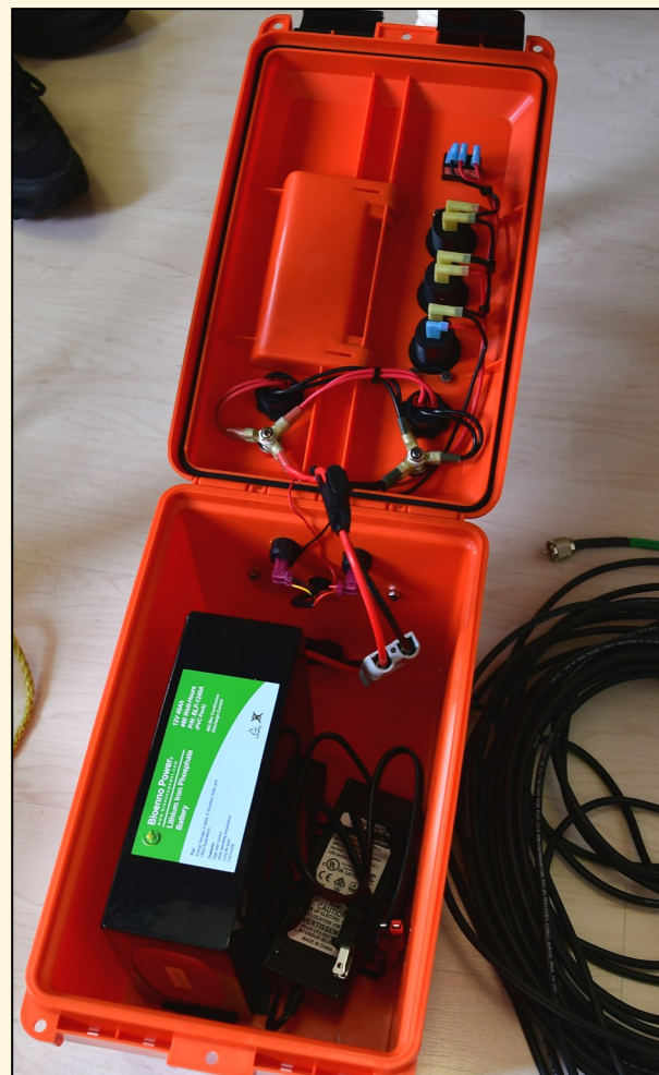
Above: A 40 Amp-hour lithium iron-phosphate battery being set up under the kitchen table for 2020 home Field Day operation entirely on portable power. PHOTO: DIANA FEINBERG, AI6DF
